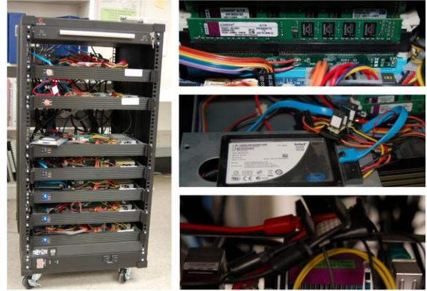
Fig. 3. The test platform (Cluster and power measurement for CPU, RAM and disk).
