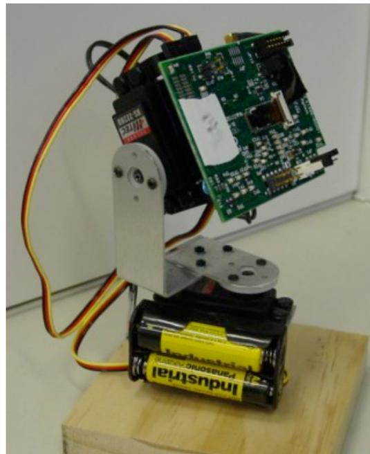
**Figure 12.** The actuation platform and pair of Mote/Cyclops. The LEDs on Cyclops are used for optical transmission of the node identity.
