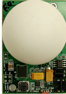
(b) Fabricated Illumimote with attachment of lumisphere
